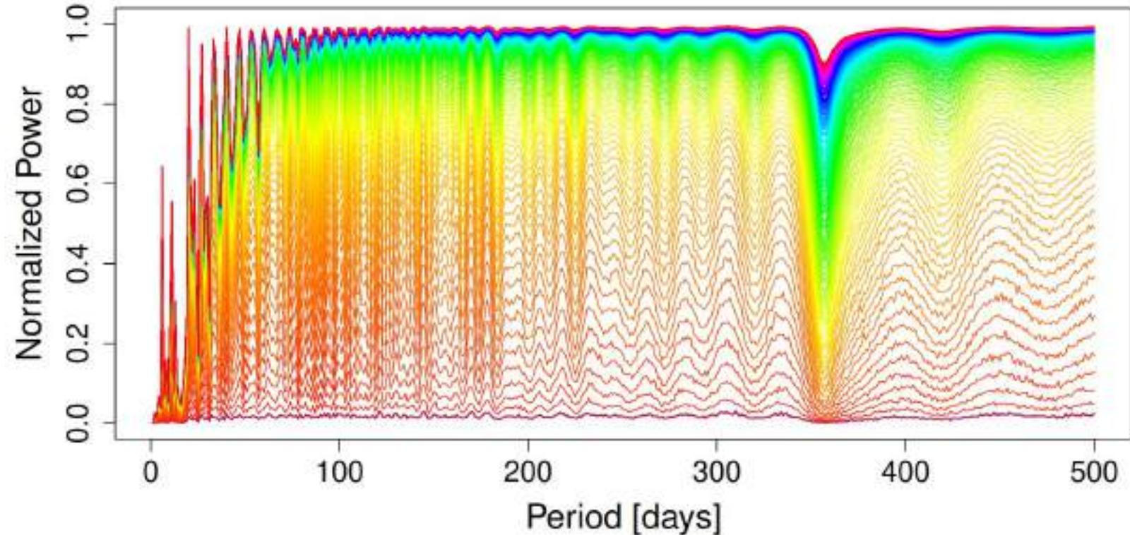
Systematic decrease of the power spectrum at some specific  $P_{\text{orb}}$  values, which is caused by the data sampling
