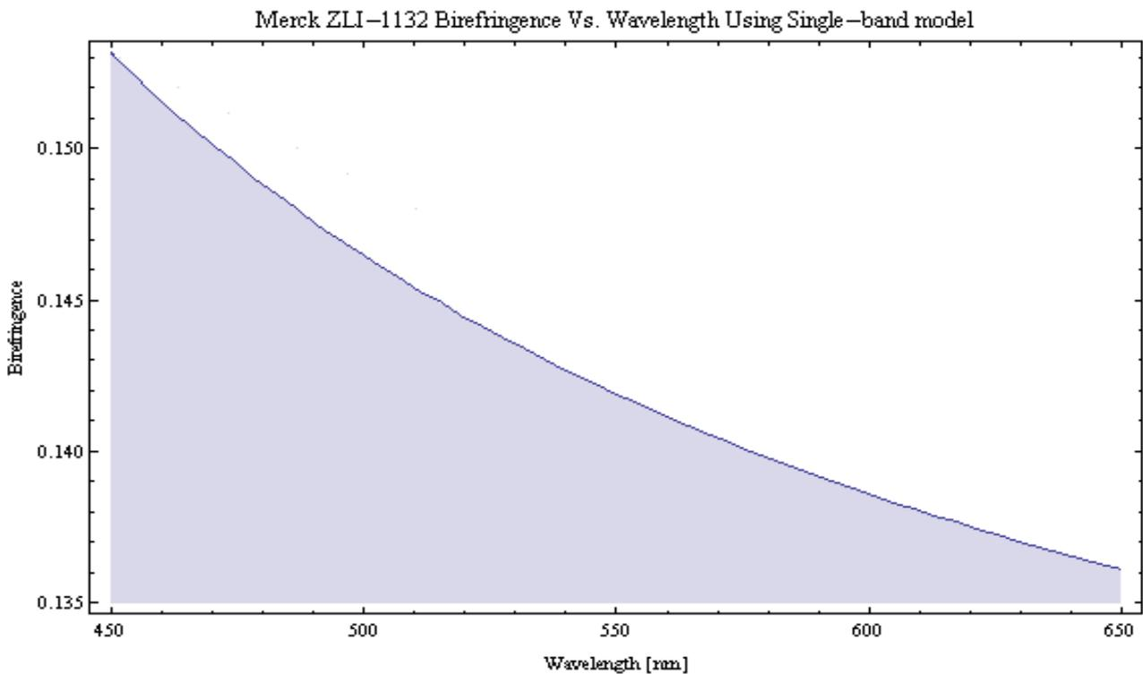
**Figure 7** - Merck ZLI-1132 Birefringence vs. Wavelength using Single-band dispersion model
