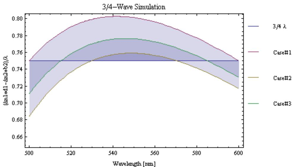
**Figure 17** -3/4-Wave Simulation using theoretical thickness
