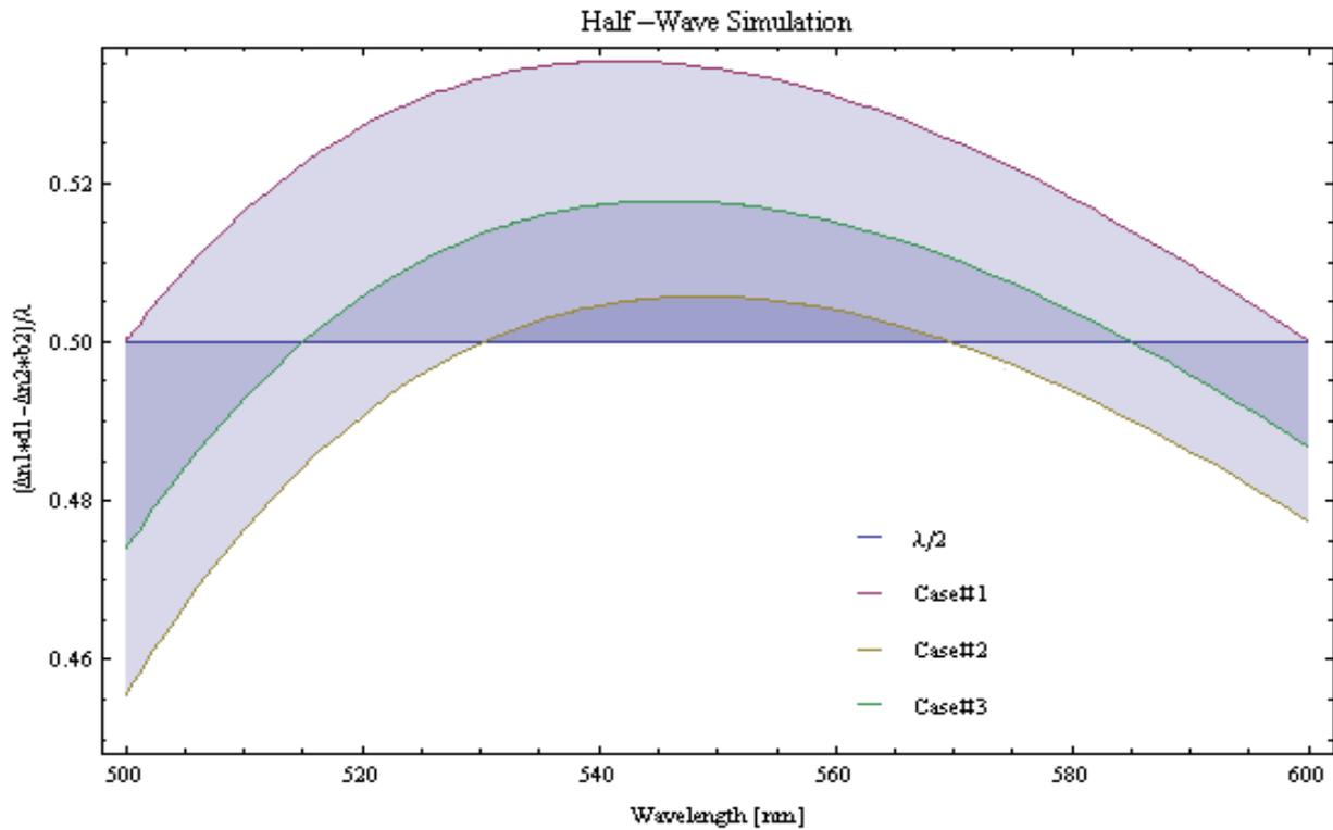
Figure 13 -Half Wave Simulation using theoretical thickness
