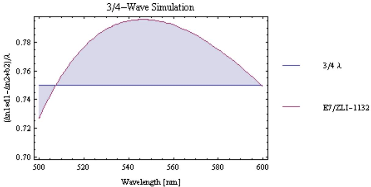
Figure 18 -3/4-Wave Simulation using thicknesses of 20 μm for E7 and 36 μm for ZLI-1132
