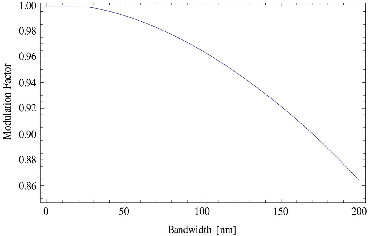
**Figure 22** -Plot of average of modulation factors ( $\mu_*$ ) vs. bandwidth for thicknesses of 10 and 20  $\mu\text{m}$
