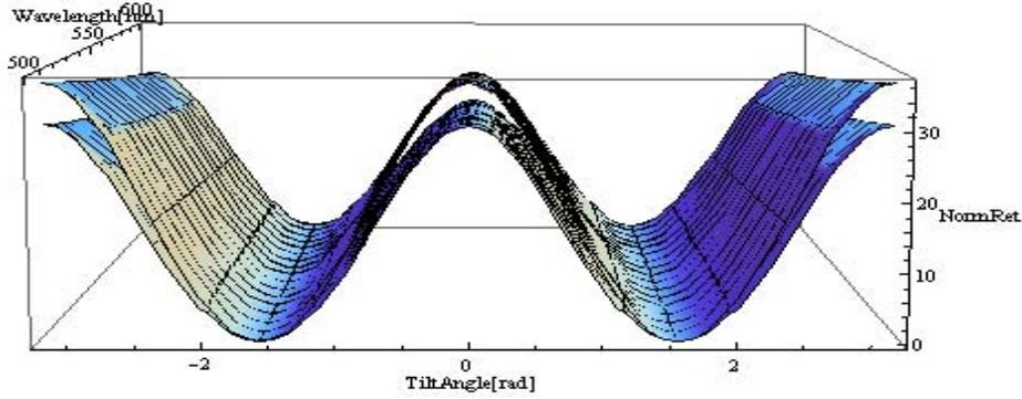
**Figure 16** - Retardances as a function of wavelength and tilt angle for E7 (upper surface) and ZLI-1132 (lower).
