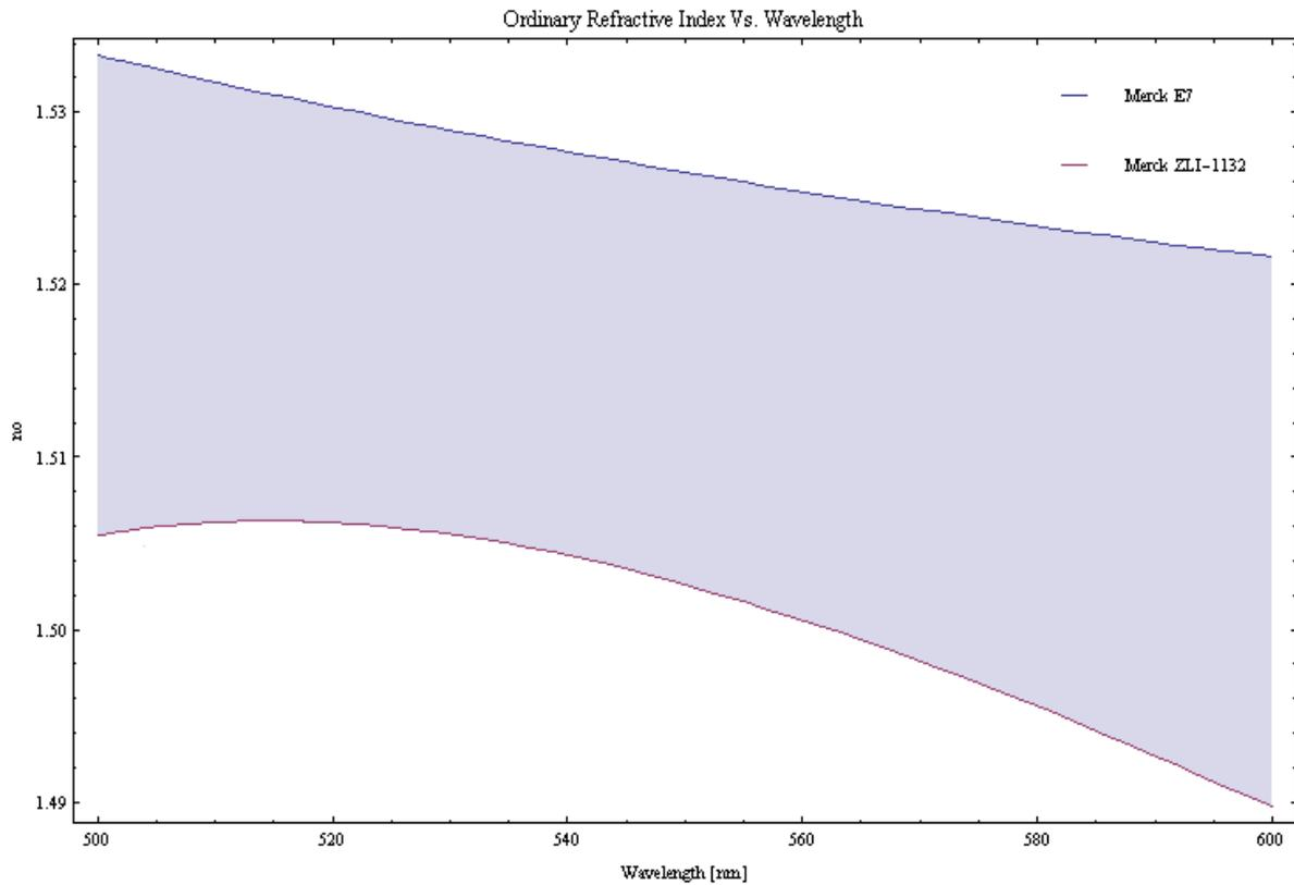
**Figure 12** -Ordinary refractive index (no) vs. Wavelength for the selected LCs
