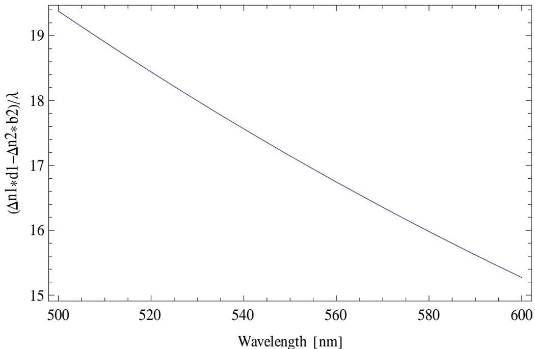
Figure 18a- Variable Retarder Simulation using thicknesses of 20 μm for E7 and 100 μm for ZLI-1132
