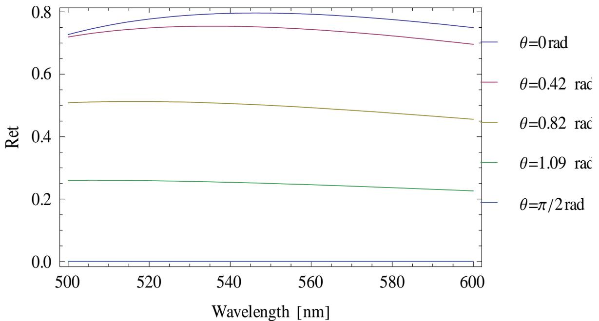
Figure 19 -Plot of effective retardance vs. wavelength (thicknesses: 20 $\mu$ m, 36 $\mu$ m)
