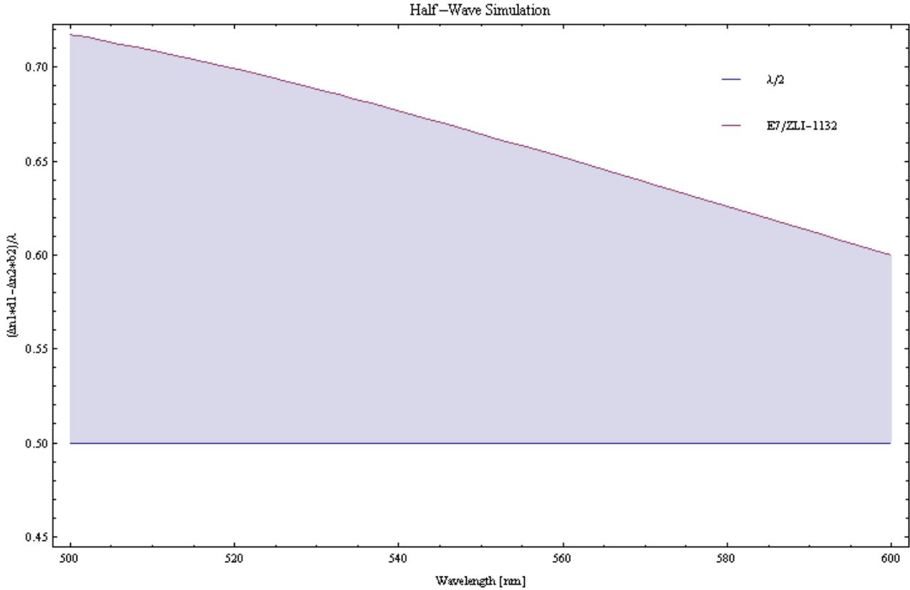
**Figure 15** -Dispersion balancing simulation using commercial thicknesses of 4.5 (E7) and 10  $\mu\text{m}$  (ZLI-1132).
