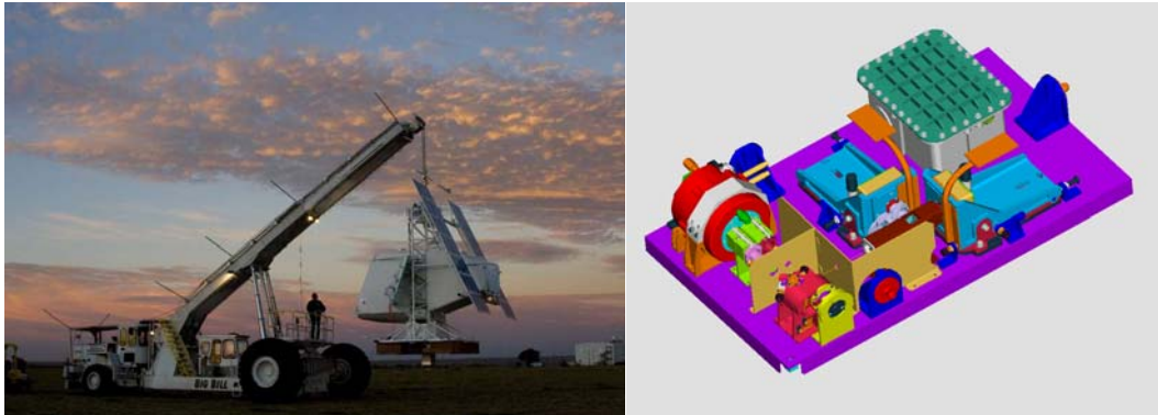
Figure 1. Left: SUNRISE test flight (October 2007), New Mexico (USA). Right: The Imaging Magnetograph; a polarimeter based on LCVRs as PMP to study the magnetic fields of the Sun
