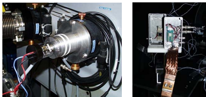
Figure 20. Deuterium lamp and flange attached to vacuum chamber, vacuum compatible UV detectors
