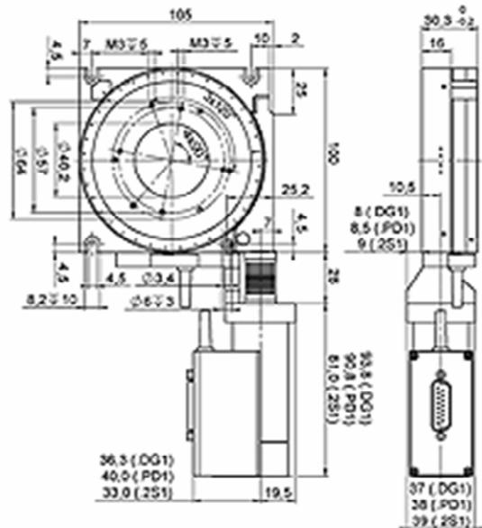
Figure 4: M-038.DG1 Rotation Stages with Worm Gear Drive (from PI Catalogue)
