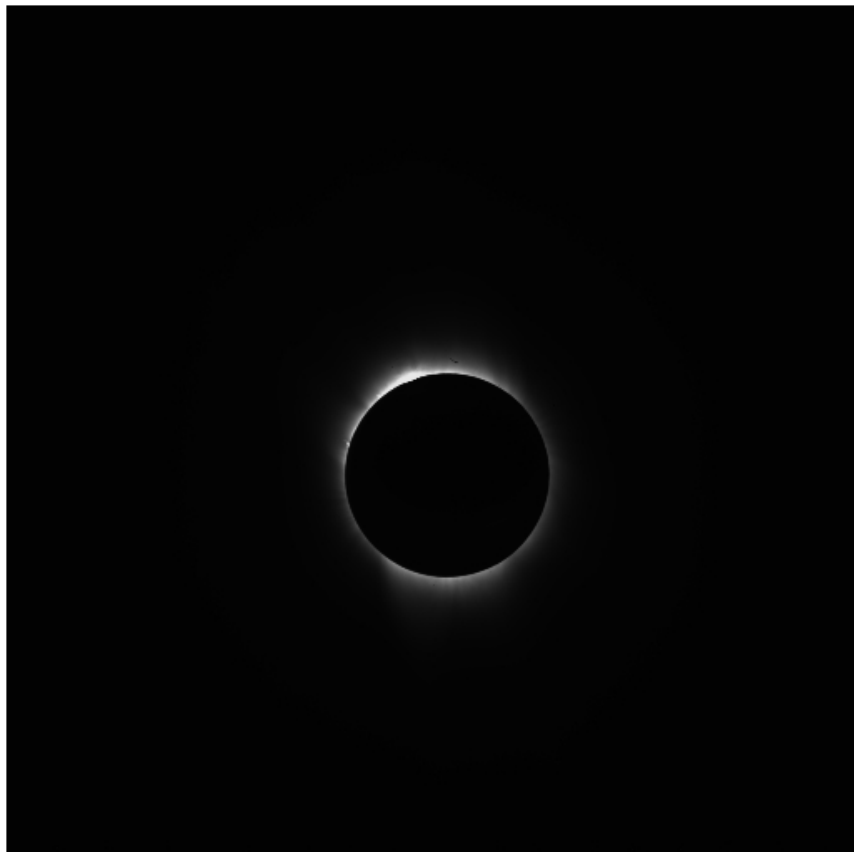
Figure 4 - Sequence #1; T_{exp} = 250 ms; V_{LCVR} = 7 V.
