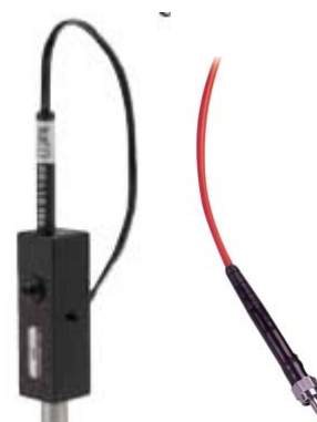
Figure 1 – Calibration Lamp mounted on a Oriel 6058 accessory with SMA adapter (left) and fiber with SMA terminator (right) [from Newport catalogue].
