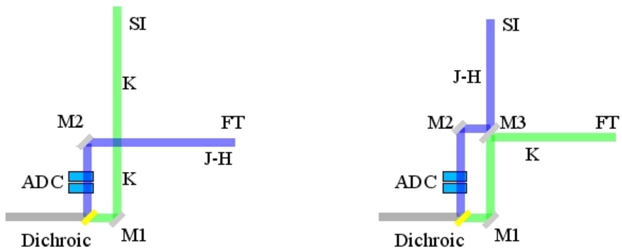
Figure 3: VSI wavelength selection configuration: H band to FT (left), K band to FT(right)
