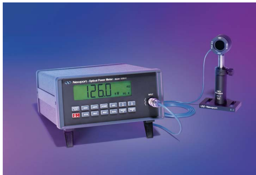
Figure B-3-4 – Optical power meter Newport 1830-C with detector [4].
